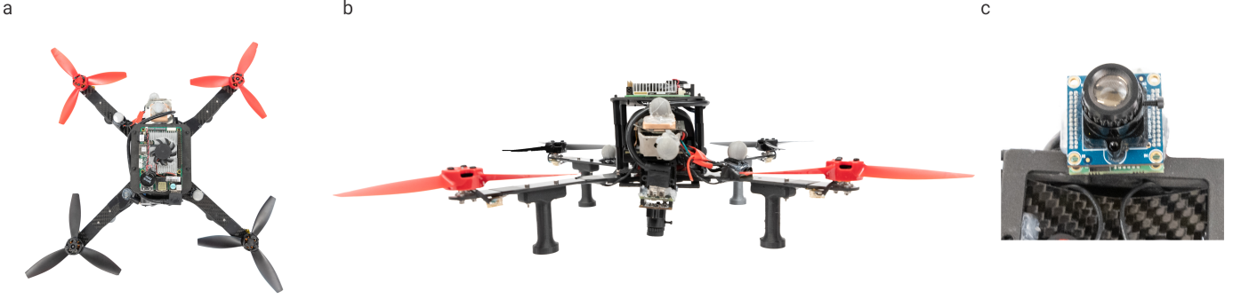
Figure 3. PRG Husky-360 \gamma platform used in flight experiments. (a) Top view, (b) front view, (c) down-facing leopard imaging camera.
