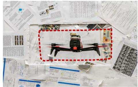
Figure 14. Quadrotor traversing an unknown window with a minimum tolerance of just 5cm. (red dashed line denotes  $\mathcal{C}$ .)
